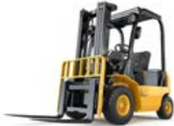
**Fig. 1 Counterbalance lift truck**
